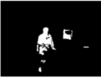
Figure 5: image subtraction reveals changed regions where the person occludes the background and at the door and a CRT.
