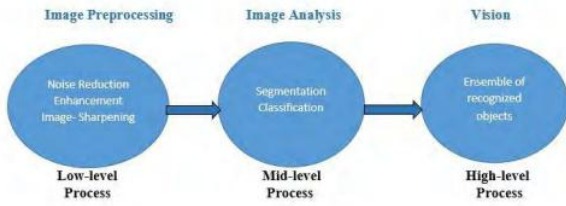
Figure 1: Low level, mid level and high level phases of Digital Image Processing
