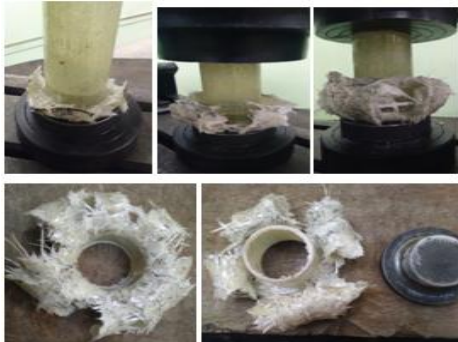
Figure 9: Deformation of tube with single radius die
