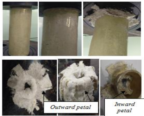
Figure 8: Deformation of tubes by flat platens without die
