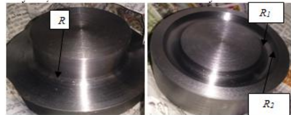
Figure 2: (a) Single radius die (b) Double radius die
