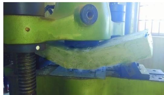
Fig 1: Metallic fibre reinforced slab
