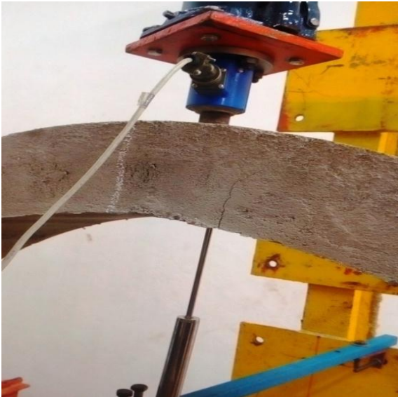
Fig 8: Initial cracks on arch
