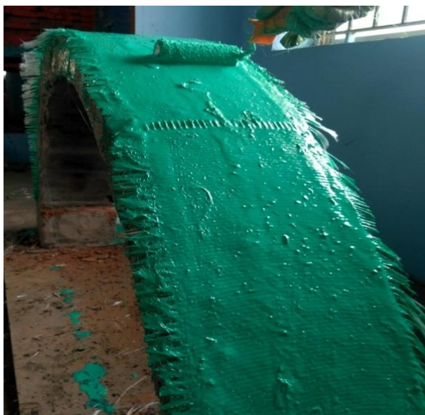
Fig 5: Application of GFRP on extrados
