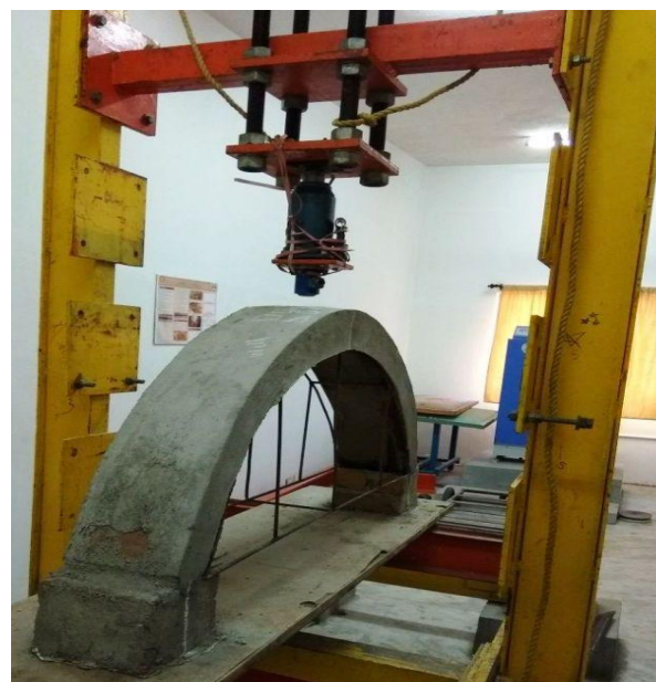
Fig 7: Loading Frame & Hydraulic jack attached to arch
