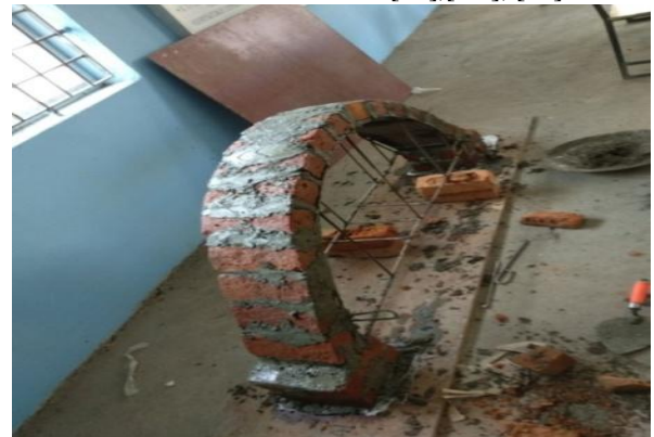
Fig 3: Casting of brick arch
