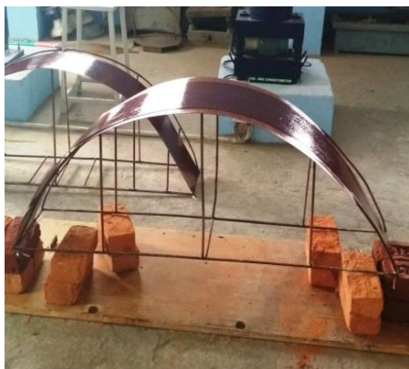
Fig 1: Preparation of steel mould
