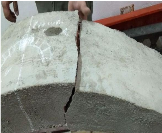
Fig 9: Major crack on arch
