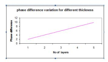
Table 1 shows that for various values of  $\alpha$  intensity transmitted through the analyzer is not uniform, there is a random variation in the intensity. At an angle of 45 degree intensity transmitted is high. For various thicknesses the phase difference is calculated and is given in table 2. The graph is plotted for phase difference variation for different thickness, it shows a linear variation between them.
