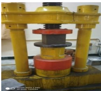
Fig 2: Compression Test of cube specimen
