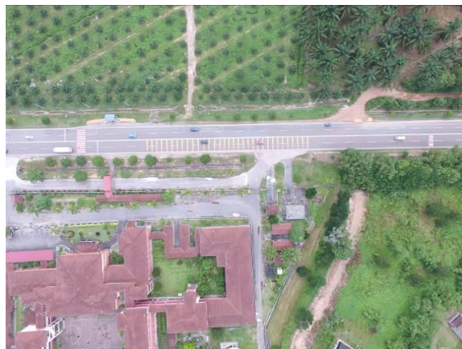
Fig. 2 Aerial view of the HPT rumble strips on the Kluang bound stretch (captured by the UAV at the height of 120 meters from ground).
