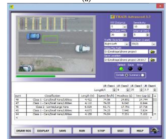
Fig. 6 Interfaces of image processing software during data extraction. (a) Downstream left lane, (b) Downstream right lane.
