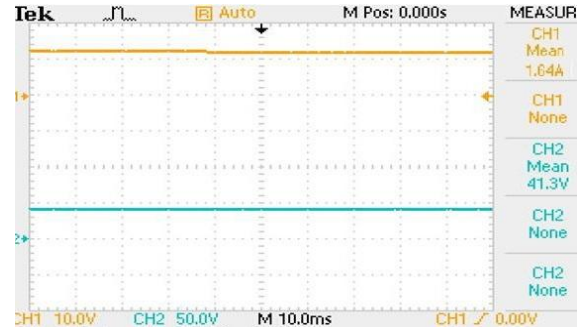
Fig 9 The load voltage and load current waveforms
