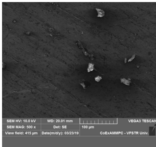
Fig: 6- 5wt% of Si 3 N 4 powder in Al 6061 alloy from SEM
