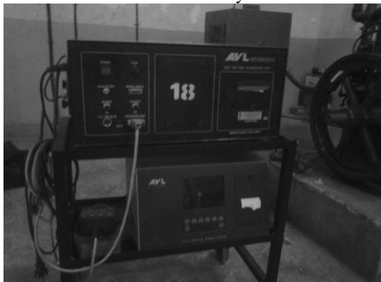
Figure 3(a) Smoke meter
