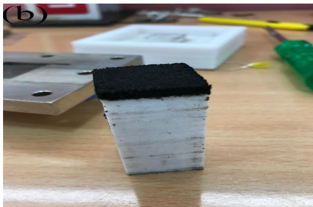
Fig. 2(b): Mould with cavity filled with slurry mixture to obtain desired shape
