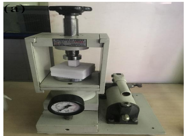
Fig.2(a): Hydraulic press used to press the mould
