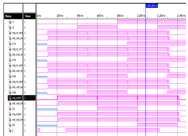
Figure 8(f): Asynchronous Simulation Wave for XOR Application.
