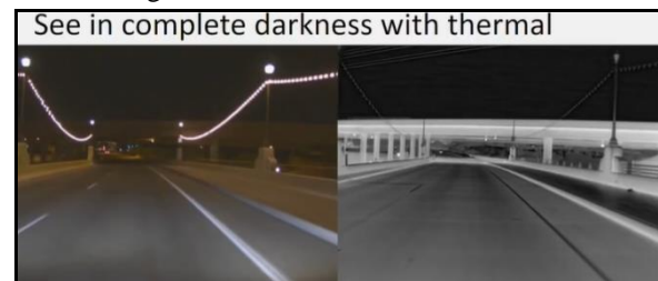
Fig. 5. Clarity of view through thermal camera
