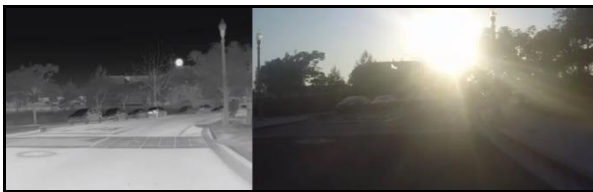
Fig. 8. Thermal not blinded by the sun
