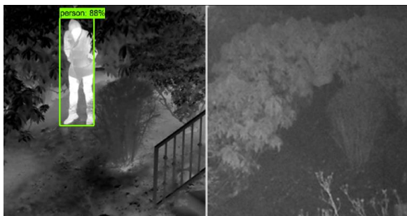
Fig. 18. Deep Thermal Imaging output-II v/s visible imagery comparison where one person is detected fully hidden in vegetation(visible imagery).
