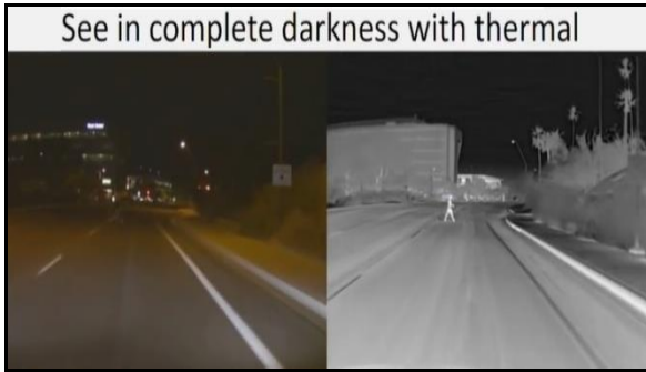
Fig. 6. Clarity of view through thermal camera
