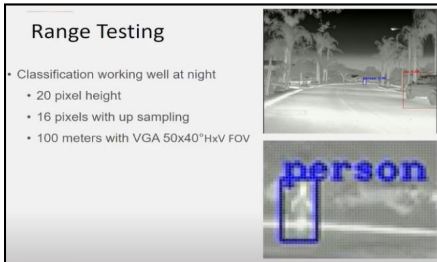
Fig. 21. Thermal camera long range testing
