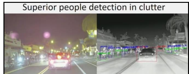
Fig. 20. Superior people detection in clutter [Visible imagery v/s Thermal imaging]
