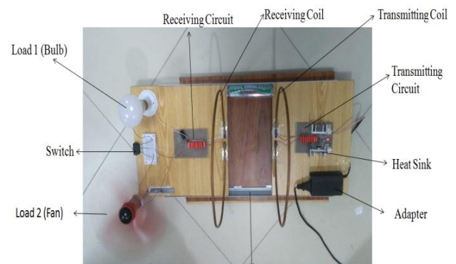
6 inches spacing Fig. 6. Transmitting Coil
