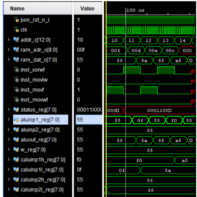
Fig. 9: 16-bit XOR operation on original core
