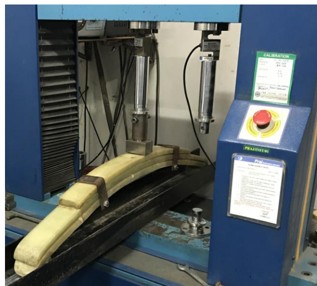
Fig. 7 Compression Test on GFRP Leaf Spring
