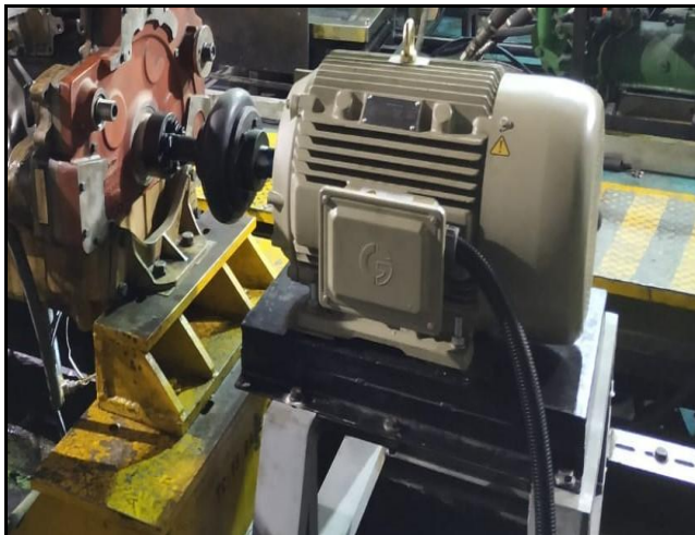
Fig. 4. Motor installed in test rig
