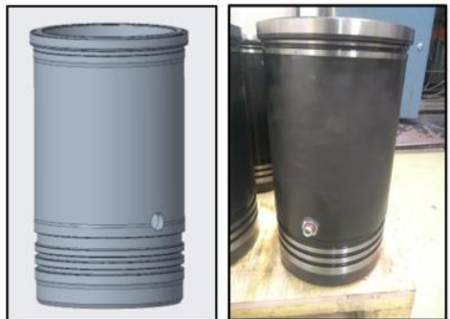
Fig.6. Modified cylinder liner
