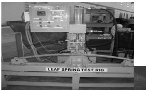
Fig. 6. Static load test for steel cart spring
