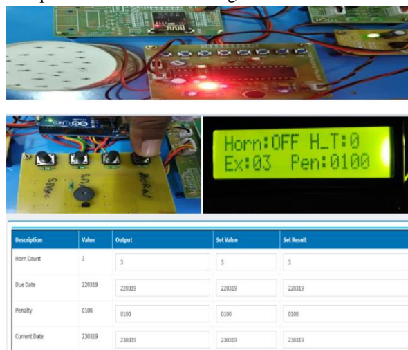
Fig. 6 Output when Horn limit exceeded
