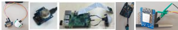
Fig. 19 (a) Interfacing and testing ; PIR, and MQ smoke, Temperature and light levels sensor
