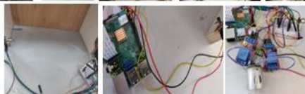
Fig. 19 (f) Subsystems testing ; car detection, gate open/close motion and safety circuit
