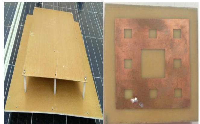
Fig.4: Fabricated Microstrip Patch Antenna element as an iteration 0(left) and Fabricated Prototype of the square Sierpinski carpet fractal antenna (right)
