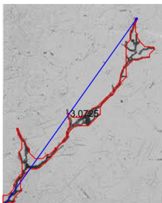
Fig. 8. Final output showing crack length
