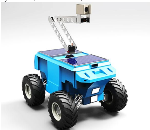
Fig. 3. Robot platform with wireless inspection camera
