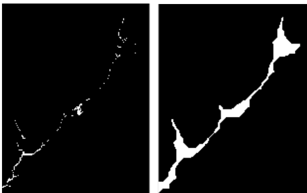
Fig. 7.(a) After threshold application (b) image after application of median filter
