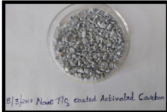
Fig 1: Activated Carbon coated with TiO 2 nanoparticles
