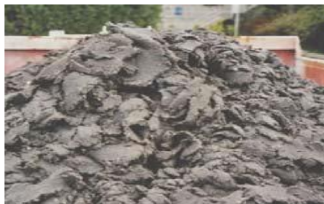
Fig. 6. Sludge after anaerobic digestion and drying.
