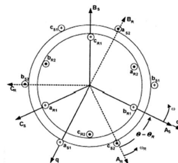
Figure 5: Asynchronous winding diagram
