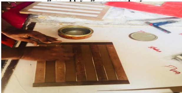
Fig. 4: Applying PVA Coating on Mold
