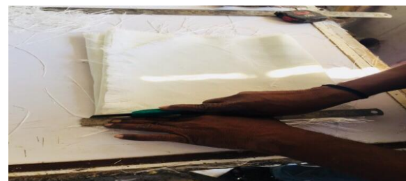
Fig 2: Cutting of Glass Fiber
