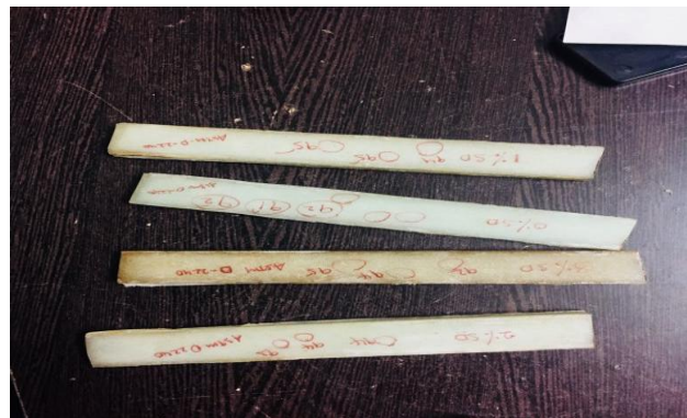
Fig. 8: Specimen for Hardness Test
