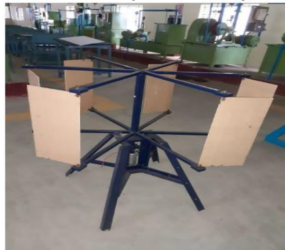
Figure 6. Final assembly of the turbine
