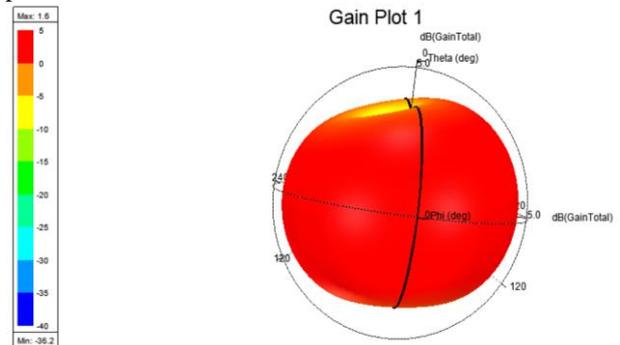
**Fig. 4. Omnidirectional radiation pattern with gain variation.**
