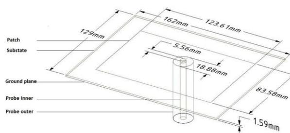
Fig. 2. Dimensions of the planar microstrip patch antenna.
