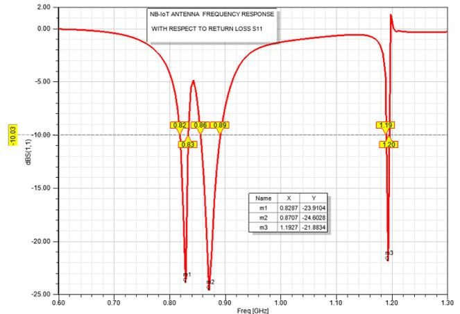
**Fig. 3. Frequency response wrt to return loss s11 in dB.**
