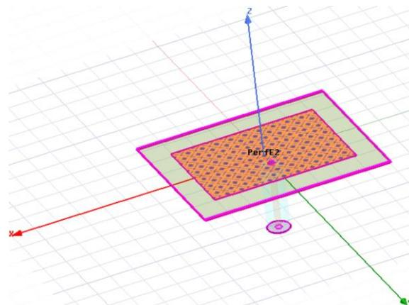
Fig. 1. Planar microstrip patch antenna.
