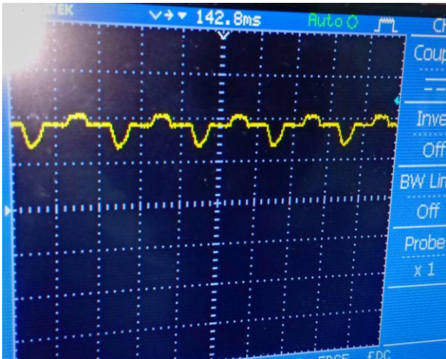
Fig 3: Nonlinear load waveform
