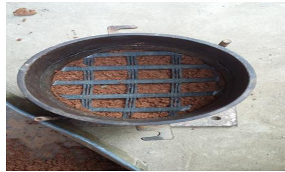
Fig: 4 Compaction of soil with geogrid layer
