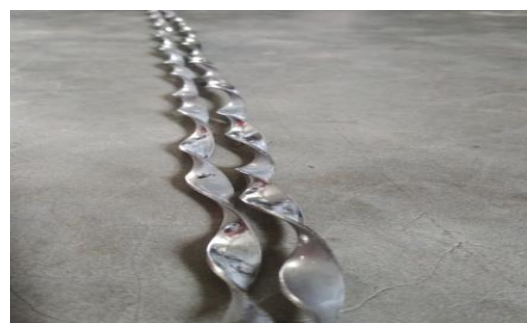
Fig. 1: Photographic view of perforated co-swirl twisted tape
