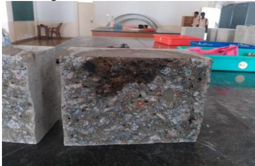
Figure Number 5.4: Chloride ion penetration test showing the penetration pattern
