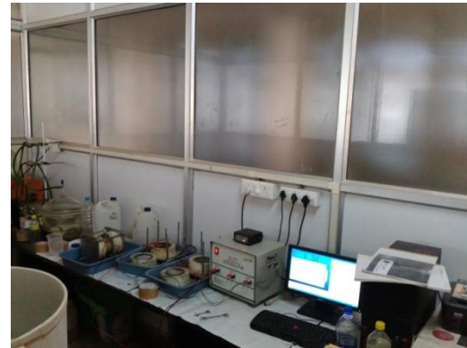
Figure Number 5.1: Total RCPT arrangement.
