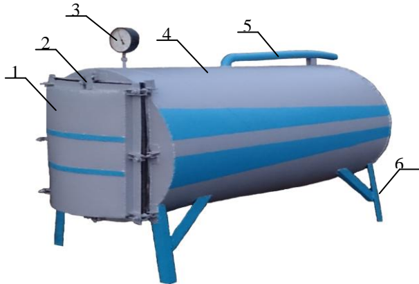
1-door vacuum chamber; 2-locking doors; 3-gauge; 4-case vacuum chamber; 5-steam outlet pipe; 6-post
