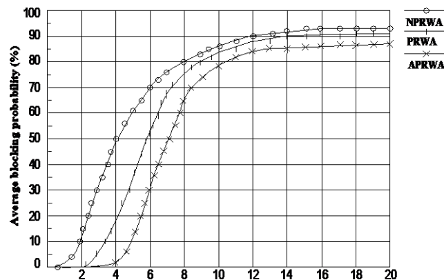
Fig. 3. Blocking probability vs traffic load for different algorithms
