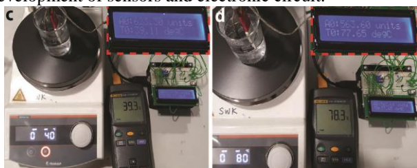
Figure 8, Experimental set up for measuring temperature. Reproduced from Sen Wai Kwok et al. [12]
