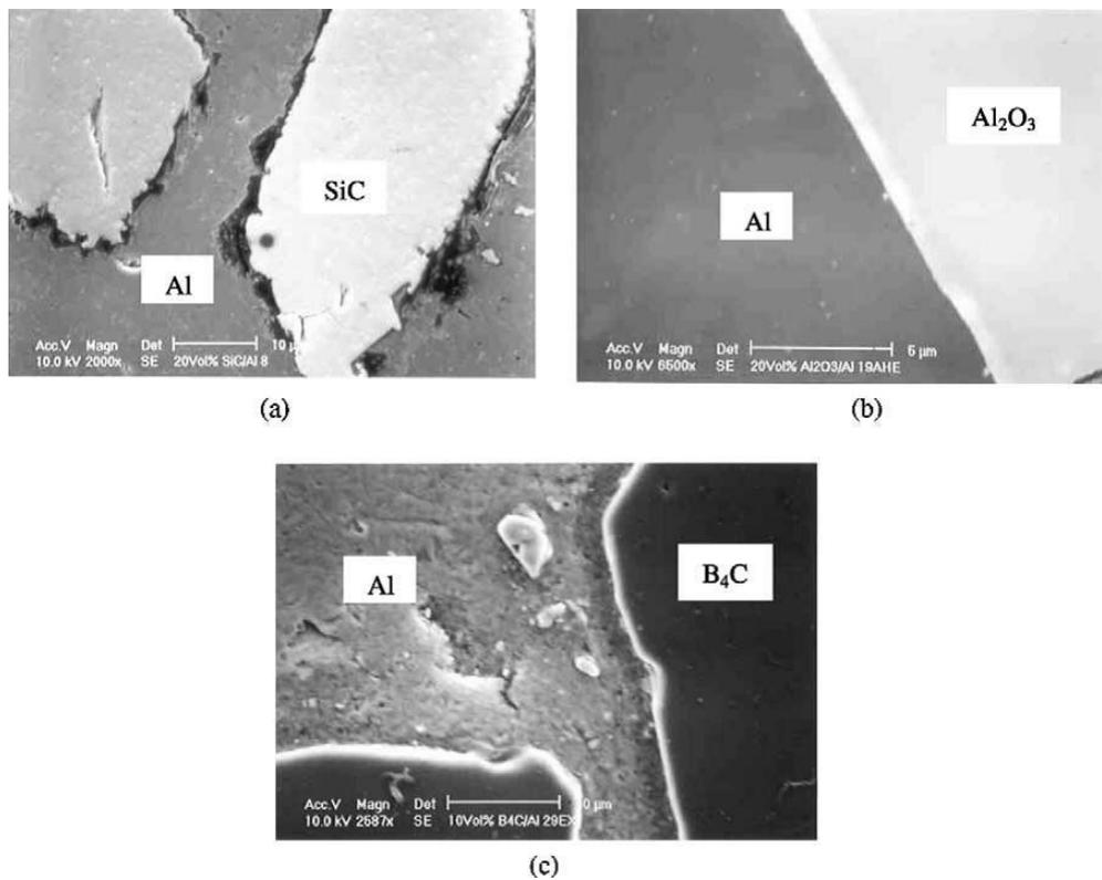
Fig. 5. SEM micrographs showing the interfaces of (a) Al/20 vol.% SiC (interaction time 60 min), (b) Al/20 vol.% Al<sub>2</sub>O<sub>3</sub> (interaction time 66 min) and (c) Al/13 vol.% B<sub>4</sub>C (interaction time 46 min) [10].
