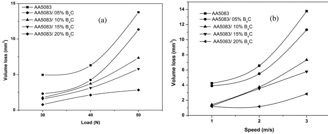
Fig. 3. Effect of (a) load, and (b) speed on volume loss of AA5083/B<sub>4</sub>C Composites [28].
