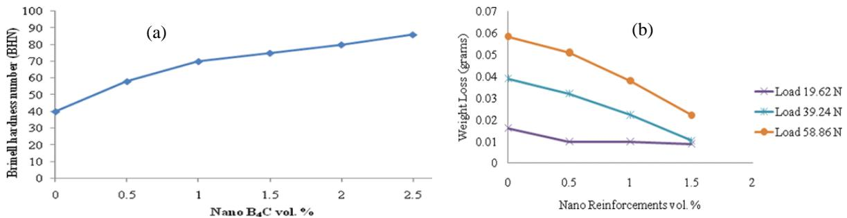
Fig. 4. Effect of nano-B<sub>4</sub>C particle reinforcement on (a) hardness and (b) wear of AA6061/nano-B<sub>4</sub>C composite [15].
