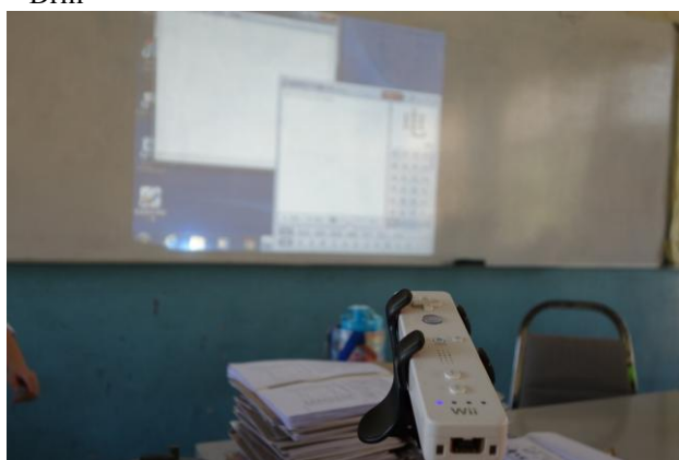
Figure 2. Screenshot of the setup and design of teaching and learning to write Chinese character using improvised low-cost Wiimote IWB
