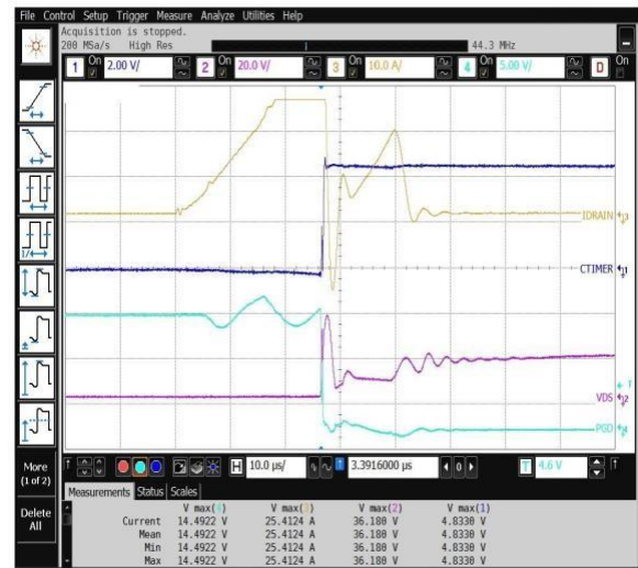
Fig 13: OR-ing FET controller shutting off QB in reverse powered condition
