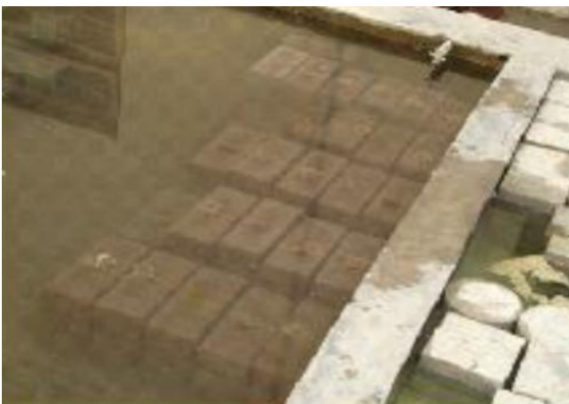
Fig. 2. Water absorption test in the site
