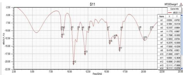
Fig 6: Return loss of Modified Antipodal Vivaldi antenna
