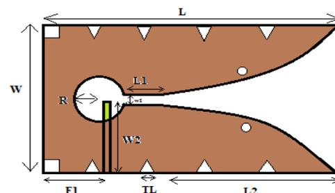
Fig 4: Design parameters of modified Antipodal Vivaldi antenna.
