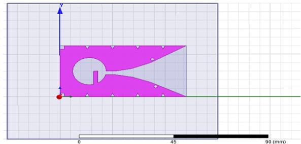
Fig 2: Modified Antipodal Vivaldi Antenna
