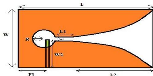
Fig 3: Design Parameters of conventional Antipodal Vivaldi antenna
