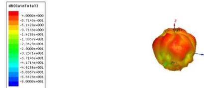
Fig 9: Gain of Conventional Antipodal Vivaldi Antenna
