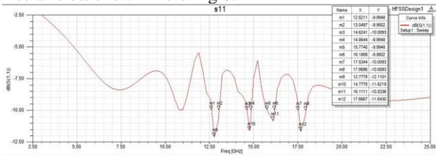
Fig 5: Return loss of conventional Antipodal Vivaldi antenna.
