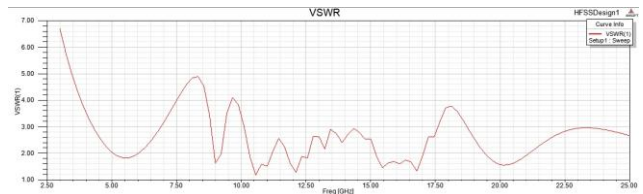
Fig 7: VSWR of conventional Antipodal Vivaldi Antenna
