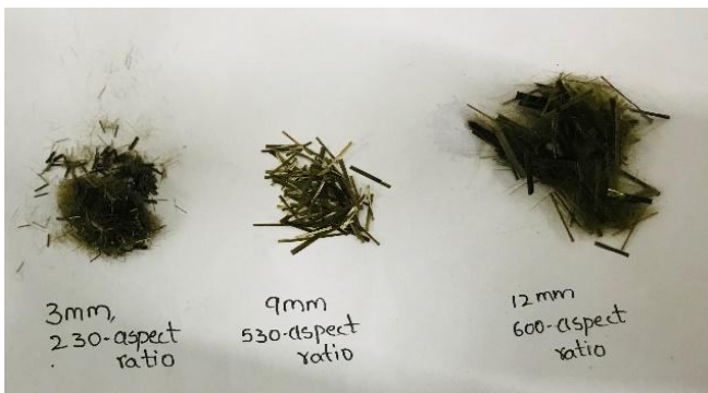
Fig. 1. Basalt fibers of length 3 mm, 9 mm and 12 mm with aspect ratio 230, 530 and 600 respectively.
