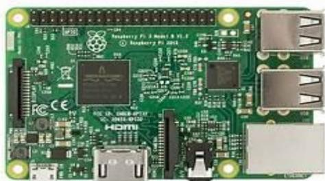
Fig. 4.Raspberry Pi 3 b Module
