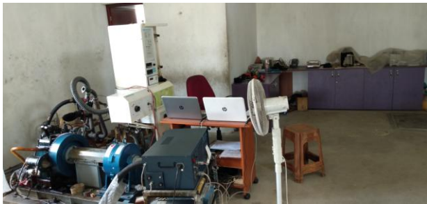
Figure 2: Kirloskar Engine Variable Compression Ratio Engine.
