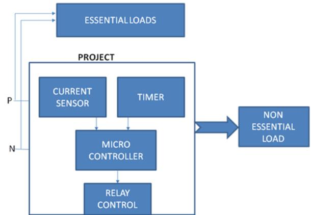
Figure 3: Block Diagram for New Houses
