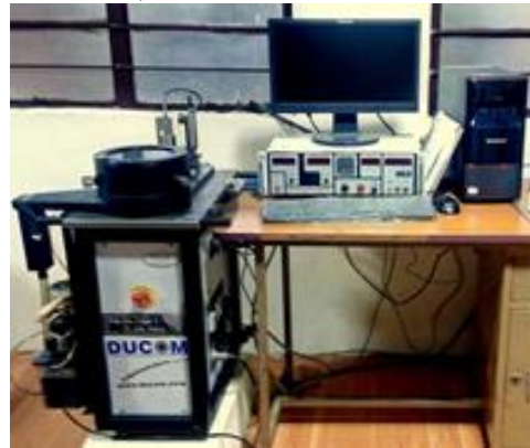
Fig. 6. Pin on Disc Machine (DUCOM – TR 20-LE)
