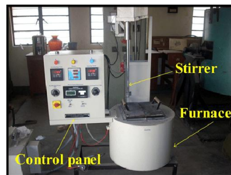
Fig. 2. Setup for stir casting process
