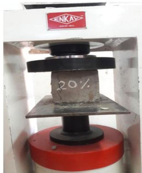
Figure: Displays compressive cube testing
