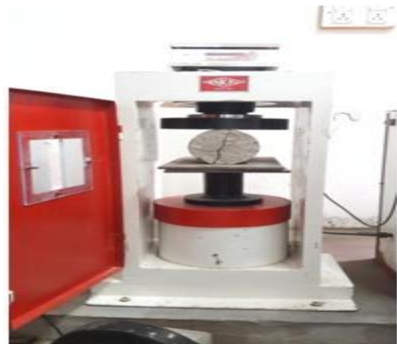
Figure: demonstrates Split Tensile Cylinder Sorptivity Test
