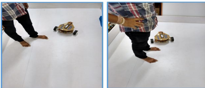
Fig. 12. (a) Navigation in an absurd non-stationary environment with a moving man hindrance, (b) Navigation in an absurd dynamic environment avoids themoving man hindrance.
