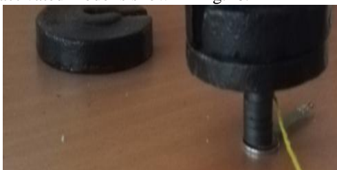
Fig. 16 – Normal load with force sensitive resistor
