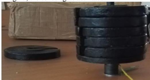
Fig. 17 – Heavy load with force sensitive resistor
