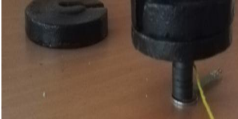
Fig. 16 – Normal load with force sensitive resistor
