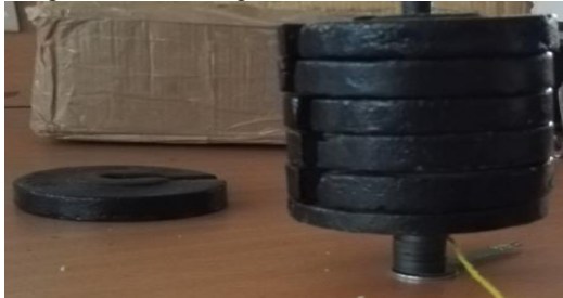
Fig. 17 – Heavy load with force sensitive resistor
