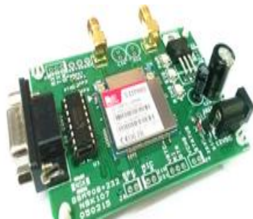
Fig. 7 – SIM 908 GPS and GSM/GPRS Module
