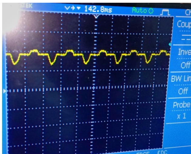
Fig 3: Nonlinear load waveform
