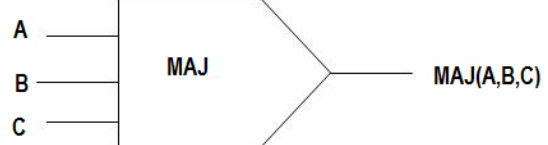
Figure 4.b: Majority gate Symbol Figure 4: Majority Gate
